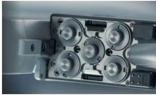
Figure 1.20: Da Vinci Xi 5-spool connector
