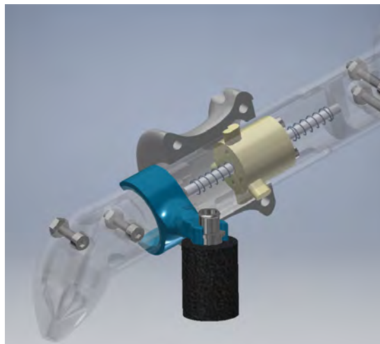
Figure 5.11: CAD image of the the catheter handle showing the cam ring (grey), followers (beige), return springs, and scope clip (blue) inside the handle (transparent grey).
