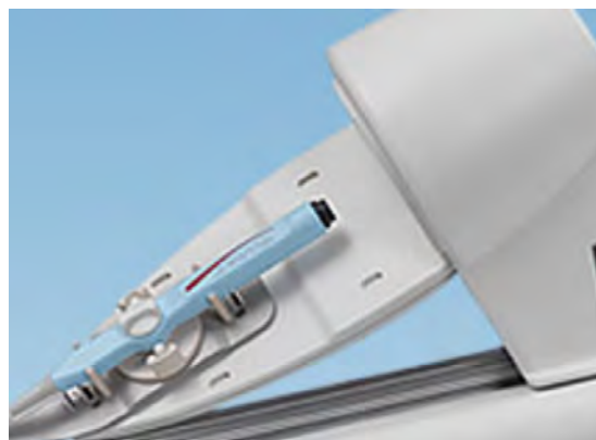
Figure 1.21: Catheter Robotics' Amigo drive element with attached Boston Scientific Blazer-series catheter
