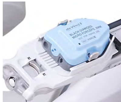
Figure 1.19: Older version Da Vinci connector system, as implemented on the Da Vinci Si.
