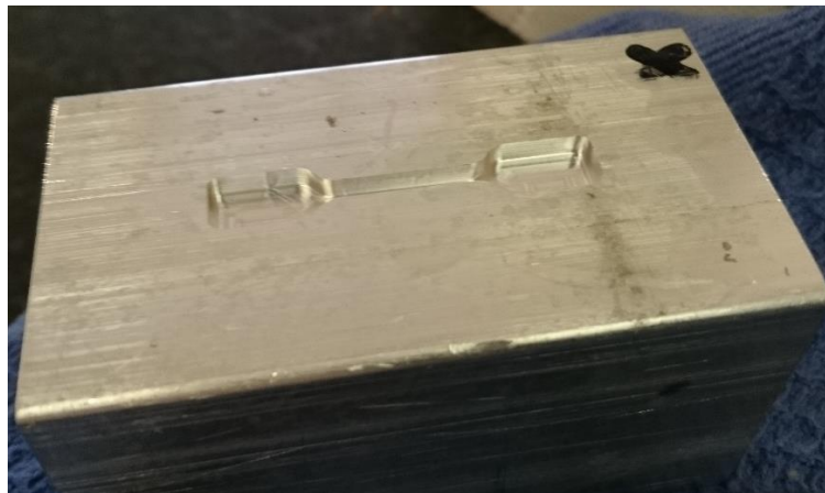
Figure 50 - mould for production of cast test pieces
