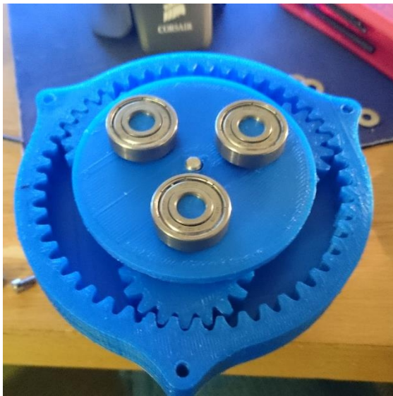
Figure 32 - Planetary gear mechanism, printed in blue PLA
