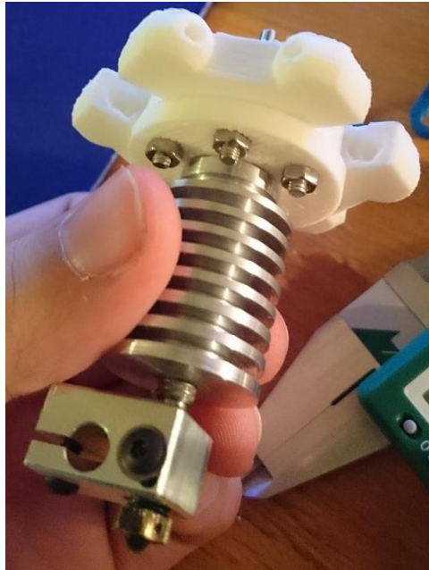
Figure 37 - modified effector plate
