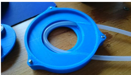
Figure 36 - lid of peristaltic pump with tubing installed
