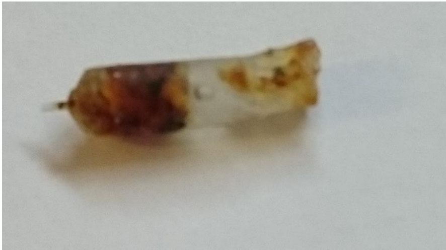
Figure 41 - degraded PVC plug
