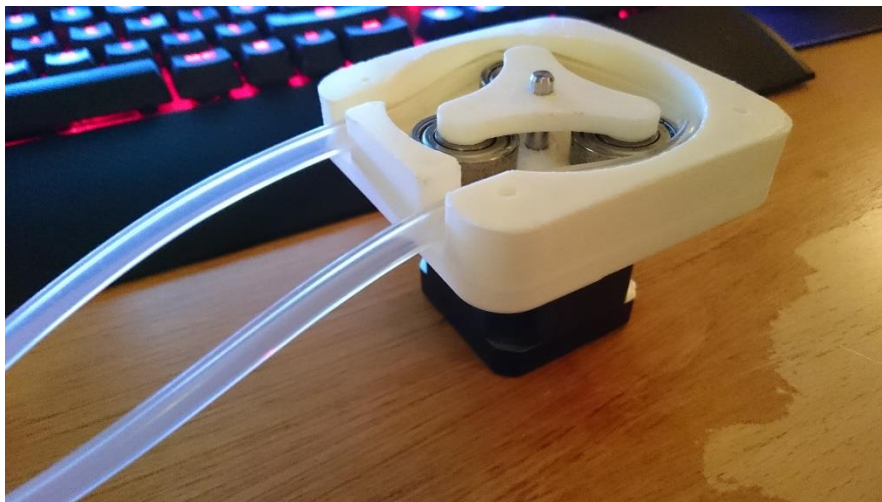
Figure 28 - 3D printed prototype, assembled with tubing and NEMA 17 stepper motor
