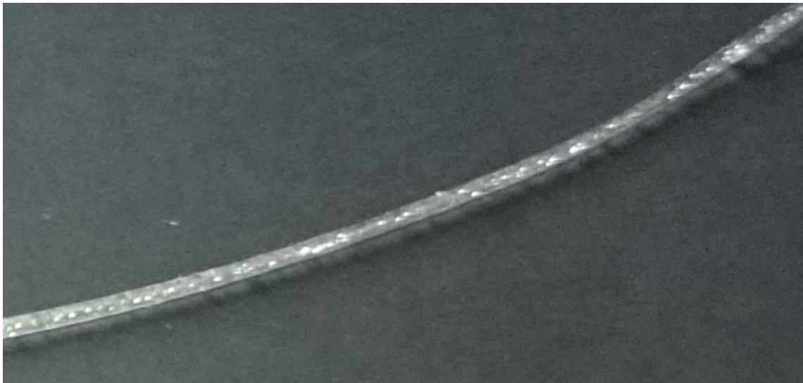
Figure 40 - extruded PVC showing air bubbles
