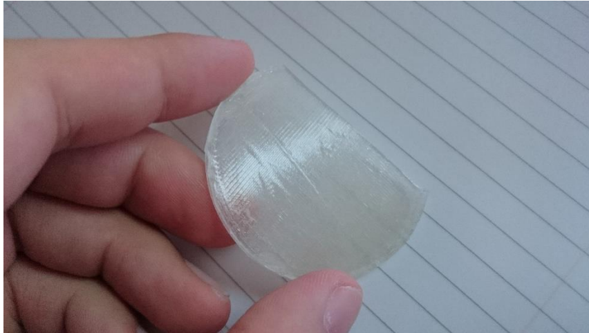
Figure 45 - 3D printed PVC puck
