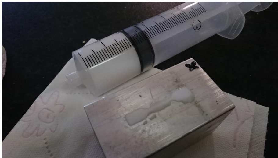
Figure 51 - filling a mould with PVC
