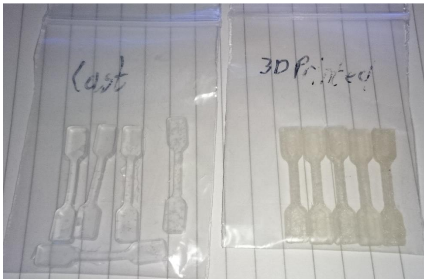
Figure 54 - Cast and 3D printed tensile testing samples side-by-side
